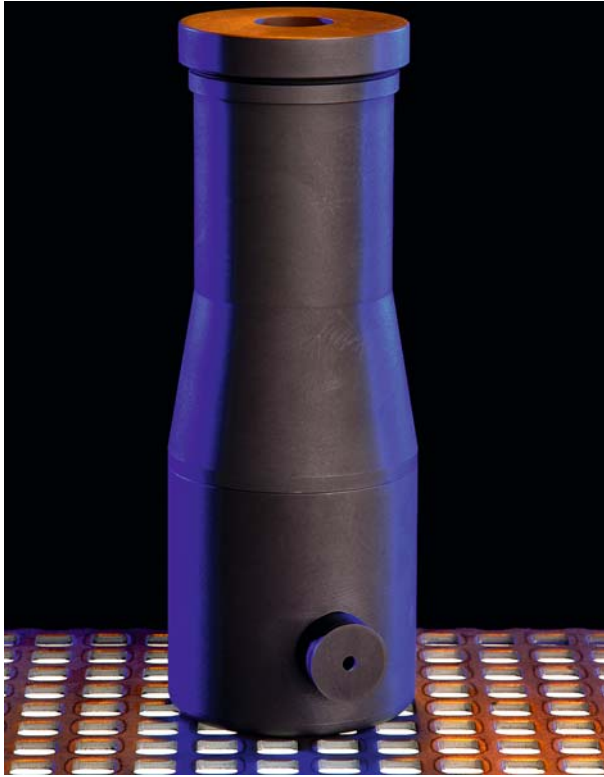
Fig. 2 Picture of the combined Ni-C eutectic fixed-point cell
